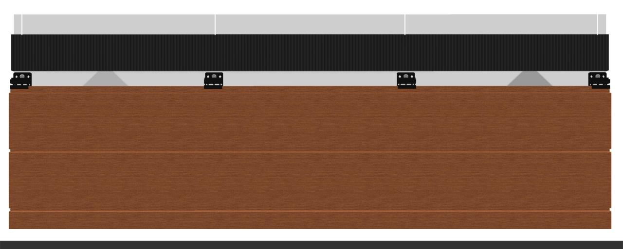
Step 12: When you are ready to install your last complete board, screw another course of Cor-A-Vent behind the board. The Cor-A-Vent will sit between your last two rows of clips.
