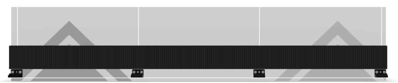
Step 6: Cut strips of Cor-A-Vent and screw into the vapor barrier/sheathing horizontally so that it fills the space between the clips. The Cor-A-Vent should run along the baseline behind your siding to permit airflow and to eliminate pests.
