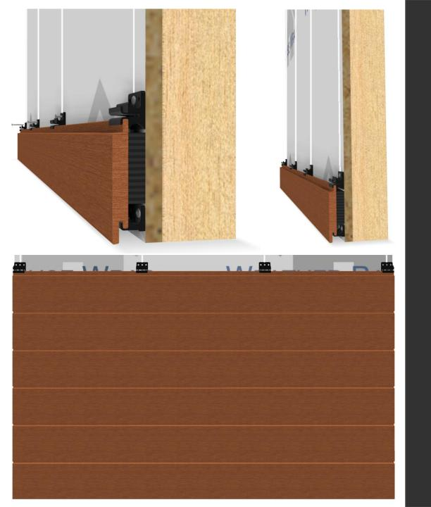
Step 9: Once the clips are engaged, install the second set of clips, driving one or two screws through the siding fastener into the stud. Ensure that the clips are level, and continue to check level throughout the installation.
