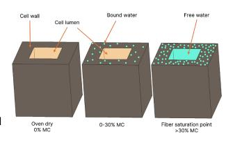
In order to make your Nova siding and decking perform the best, it needs to be acclimated to the end use environment. Acclimating is a crucial step that allows the wood to reach EMC in the environment that it will be installed in. Failure to acclimate appropriately may result in defects such as cupping, twisting, checking, fastener withdrawal, shrinking, and swelling, either before during, or after installation.
